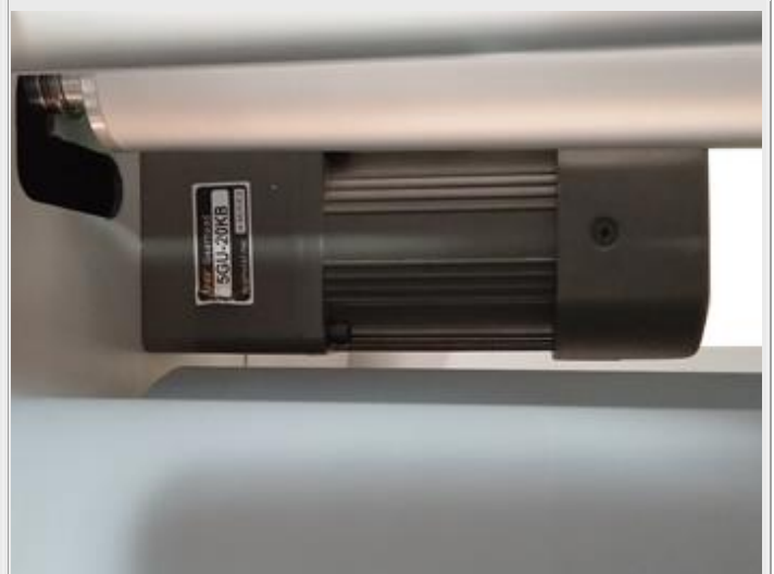
140W speed adjustable force moment motor
